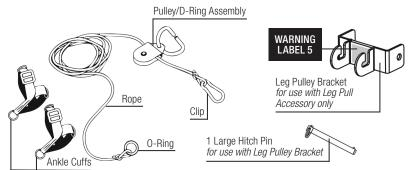
Connect the Leg Pulley Bracket to the top of the Vertical Column by aligning Bracket with the hole at the top of the column; be sure Bracket is right side up. Insert Large Hitch Pin through the hole to secure Bracket onto the Vertical Column.
