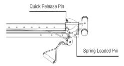
B. Take hold of the Vertical Column and pull it up until it is upright. Release the Spring Loaded Pin. You should hear it lock back into place. (NOTE: Pin is on left side.)
