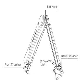
4. Make sure the Handles are out to the sides before you begin to unfold your unit. Keep hands and fingers away from Pulley. Hold onto the top center of Glideboard and begin rolling rear Tube Rollers. Spread the unit out until it is flat on the floor. Be careful to do this slowly.
