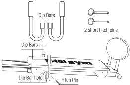
**1.** Attach each dip bar to the frame with the short hitch pins included with your Total Gym<sup>®</sup>.
