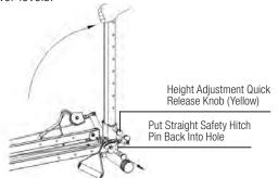
**5B.** Insert the Straight Safety Hitch Pin connected to the lanyard through the safety hole on the side of the height adjustment slide mechanism until it is through the Vertical Column. NOTE: Insert Safety Hitch C Pin into side hole located directly below Height Adjustment
