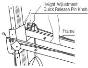
5. Pull out the black Spring Loaded Pin Knob located at the right rail. Continue to hold pin out while taking hold of the Vertical Column and lowering it forward towards the center rail & glide board. Once completely forward, velease the Pin. You should hear it snap back into place.
