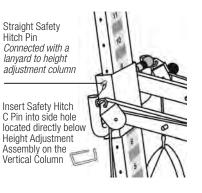
Assembly on the Vertical Column. Never sit or exercise on Total Gym without the yellow Height Adjustment Quick Release Pin Knob, Straight Safety Hitch Pin and Safety Hitch C Pin securely locked into place.
