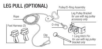
Connect the Leg Pull Bracket to the top of the Vertical Column by aligning Bracket with the hole at the top of the column; be sure bracket is right side up with hooks facing upward. Insert Long Hitch Pin through the top holes to secure Bracket onto the Vertical Column.
