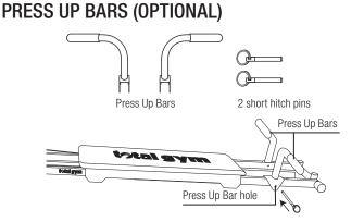
**1.** Attach each press up bar to the frame with the short hitch pins included with your Total Gym<sup>®</sup>.
