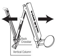
**4B. Continue to carefully lower the rails slowly,** unfolding the unit until it is flat on the floor with the Vertical Column in full upright position.
